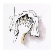
Apply at temperature range +15°C to +25°C (+60°F to +80°F). Surfaces should be clean and dry, free of dust, grease, oil and any other loose matter. Do not use degreasing products. Not for use in application likely to make contact with chlorinated, cetonic or esther solvents.
