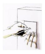
Place the hanger in the required position and press the base against the surface to be insulated
