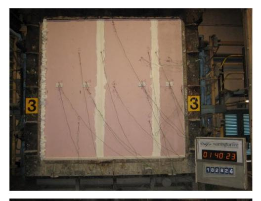
The unexposed face of the specimens after 111 minutes of the test
