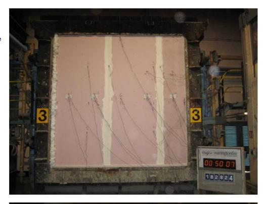
The unexposed face of the specimens after 60 minutes of the test
