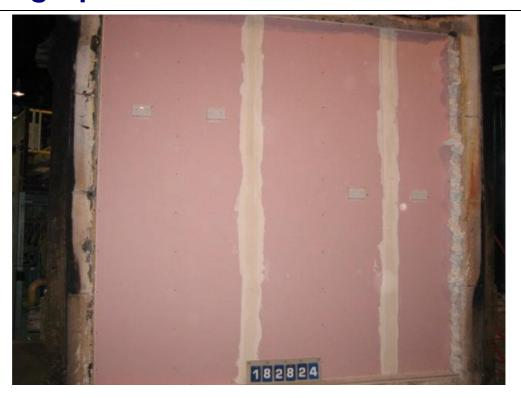
The unexposed face of the specimens after 20 minutes of testing
