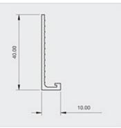
Locally manufactured from recycled plastic, Renderplas PVCu stop beads are designed for function and speed on all external and internal rendering and plastering applications. Discreet but strong, all beading gives a perfect finish to through colour render and is equally suitable for sand and cement
