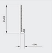
Locally manufactured from recycled plastic, Renderplas PVCu small wing stop beads are designed for economy and speed on external and internal rendering and plastering applications where the substrate is even
