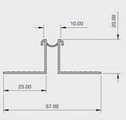
Locally manufactured from recycled plastic, Renderplas PVCu movement joint / expansion joint beads are designed for areas of render over 20 square metres and should be specified every 4-6 metres, over structural movement joints and changes of background. Discreet but strong, all beading gives a perfect finish to through colour render and is equally suitable for sand and cement
