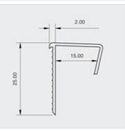
Locally manufactured from recycled plastic, Renderplas PVCu clip on edge beads / board stops are designed for plasterboard and cement board to provide protection to edges and a superior finish. On plasterboard at edges formed at door frames, windows and skirting boards or at a change of finish; on cement board at the exposed edge of the system
